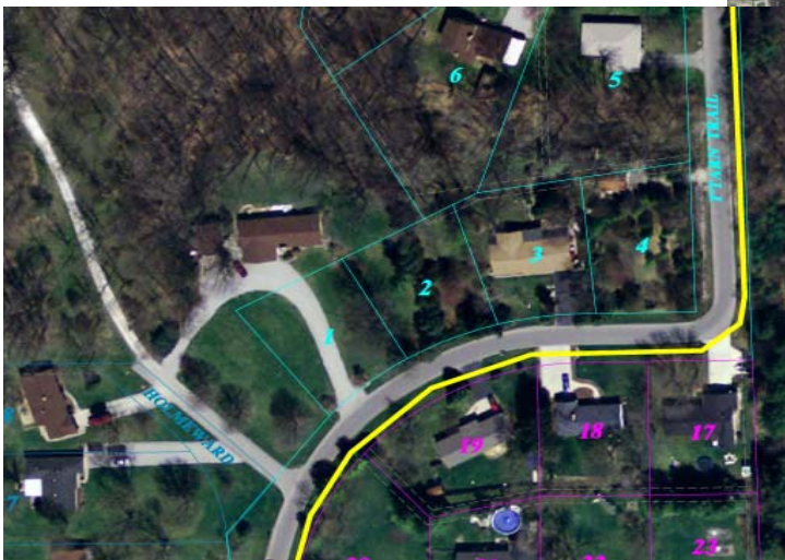
Aerial photograph with proposed Force Main alignment
